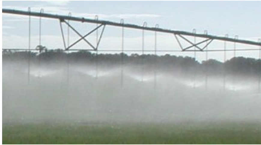
Figure 4. Wobbling diffuser (IWOB) sprinkler nozzles in operation.
