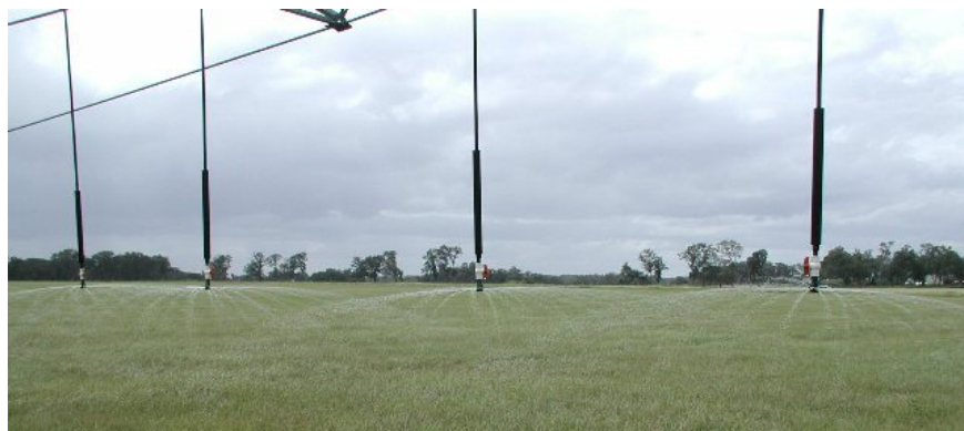
Figure 5. Single pad grooved plate low drift nozzle (LDN) sprinklers in operation.
