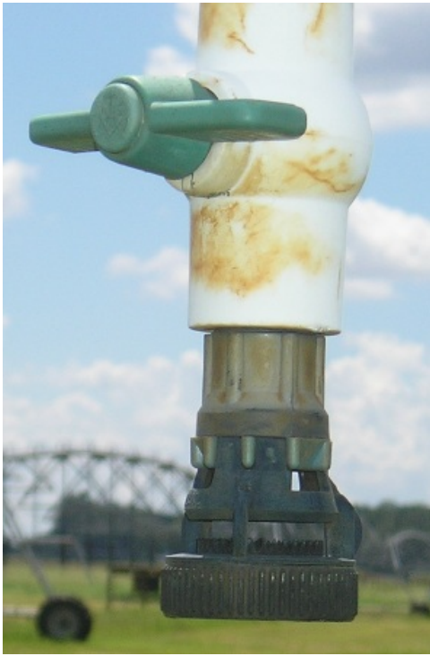
Figure 1. Single pad grooved plate low drift nozzle (LDN) sprinkler.
